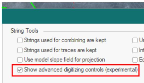
The next use of either command displays a popup allowing you to constrain the length, azimuth and gradient of the next string edge. For constrained angle changes, you can also ensure azimuth changes are made in fixed amounts from the previous string segment:
